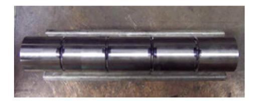
**Orifice Plates:** mounted in series - optimized plate spacing for each unit from 1D to 5D (D, pipe internal diameter). The number of stages can vary from 1 to more than 10 if required.
