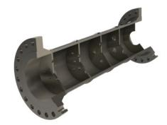
ASIAN INDUSTRIAL VALVES AND INSTRUMENTS make ASVIN MULTI-STAGE RESTRICTION ORIFICE ASSEMBLY (several Orifice Plates in series), is used if the desired pressure drop could not be achieved with a single plate. Each Orifice Plate or stage enables reducing the pressure to its maximum while avoiding the phenomena of cavitation and critical flow.
